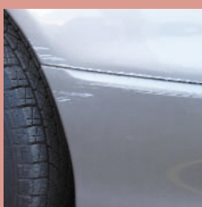
Abrasions of more than 25mm in length
